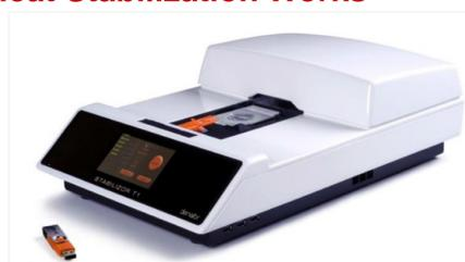
The tissue is inserted into a Maintainer Card made of thin Teflon foil that allows for rapid conduction of heat. The card is evacuated to 5-10mbar and a class 1 laser measures the size of the tissue. Two aluminum blocks come into contact above and below the tissue and the sample is heated up to 95°C and an algorithm determines the length of time necessary for complete inactivation based on sample size.
